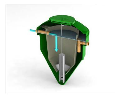
1: The wastewater flows into the main tank and enters directly into the bio-chamber.
